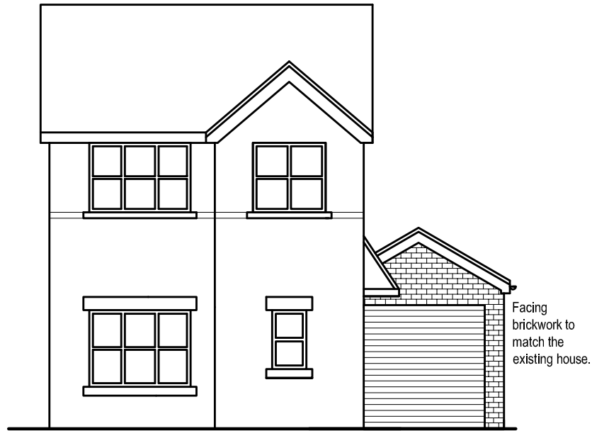
FRONT ELEVATION AS PROPOSED (1:100)
